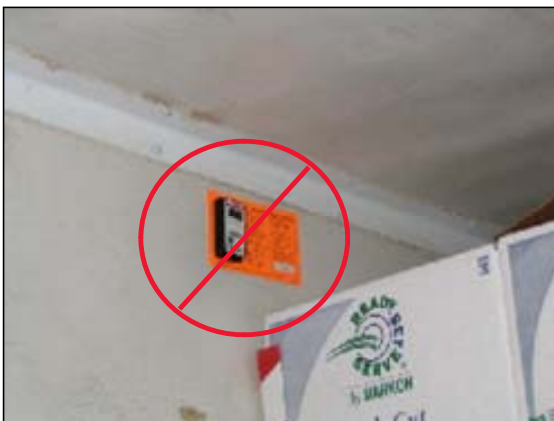
Incorrect TempTale Placement
